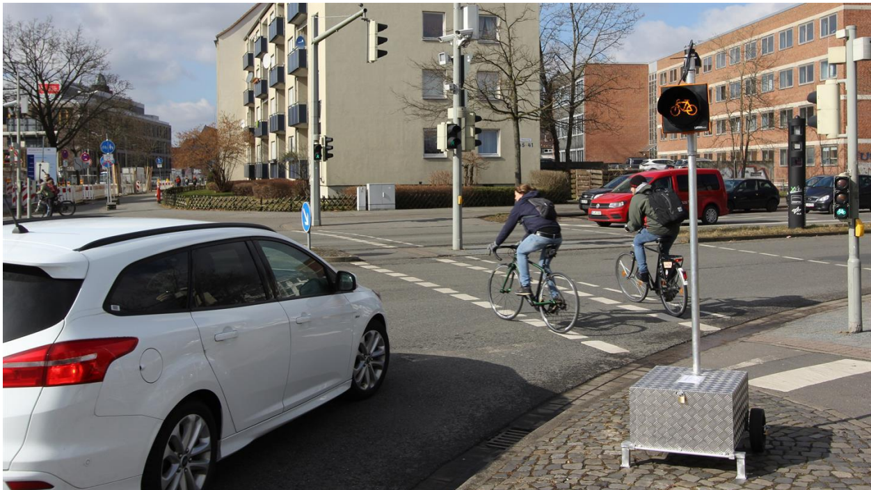
Figure 3: Installation of the amber Light at the AIM Research Intersection showing the warning for the motorist.
