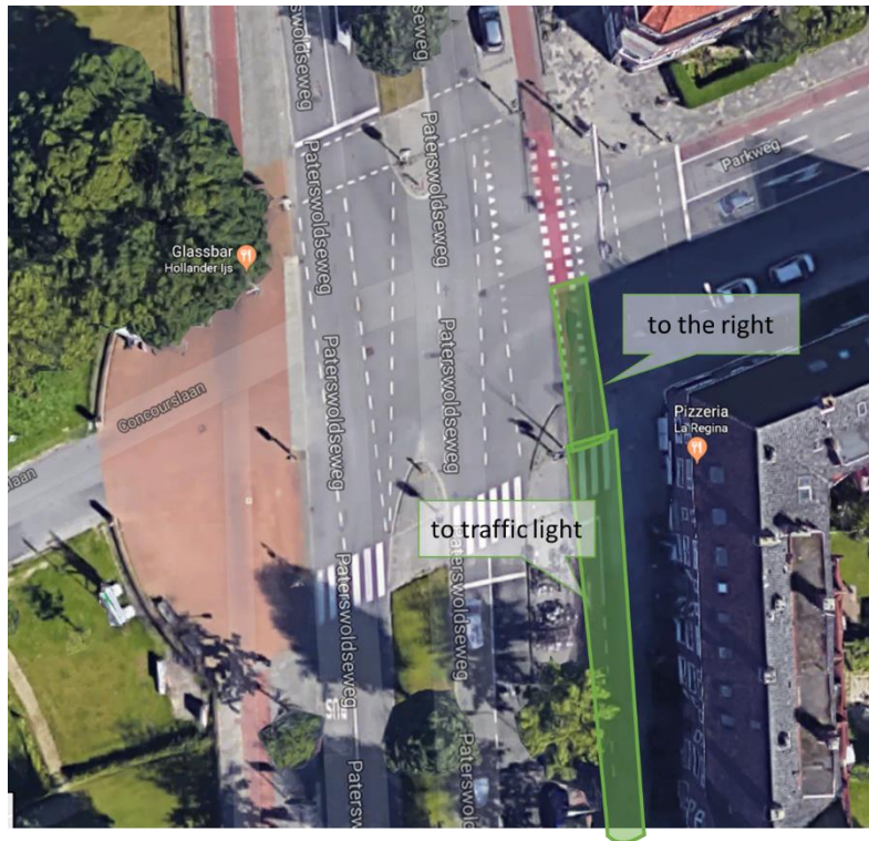
Figure 54: Illustration of the MiRA-zones “to the right” and “to traffic light”. The traffic light had to be checked before passing it, but could be done so over a longer approach area. The road to the right could first be checked for potential traffic when the house on the side was passed, and had to be done so at the latest before reaching the lane coming from the right.
