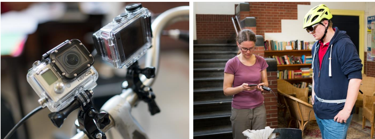
Figure 50: The bicycle of a participant equipped with the two cameras (left), and a test leader calibrating the eye tracker to one of the participants (right).
