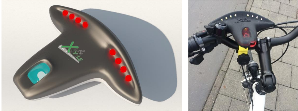
Figure 4: Left: Sketch of the designed HMI. Right: Result of the 3D printing mounted to the handlebar.
