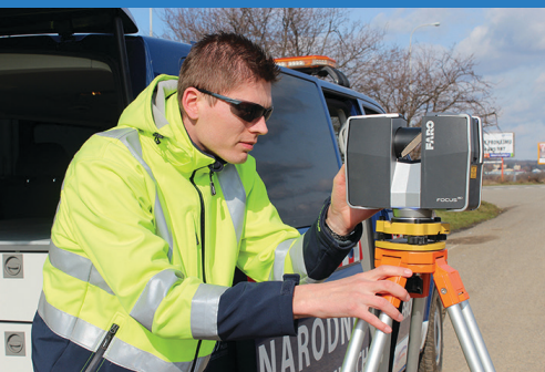
vehicle deformation scanning with the use of a 3D scanner
