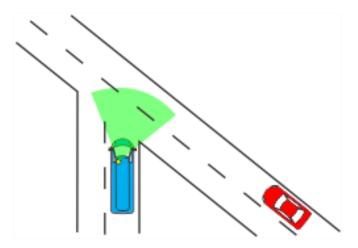
Behind, through the rear-view mirrors, the driver has visibility of approximately 15-20° on either side of the truck.
