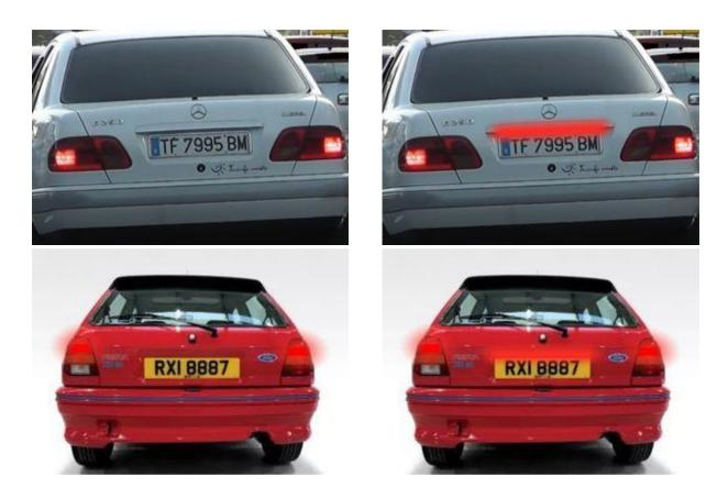
The license plate is a visible surface for any vehicle and the electrical wiring would not affect the passenger compartment, so it is the best place to locate the 3rd brake light for both old cars and commercial vehicles. Even though they are old, these cars are and will be present in traffic for a long time, especially in states where purchasing power is low.
