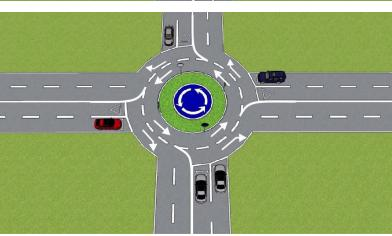
The logical solution for multilane roundabouts is for the first lane (outer lane) to be used for exit only,
