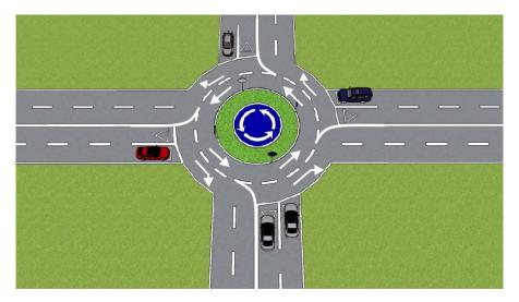
In this way, after giving priority (to those on the left) when entering the roundabout, all vehicles will exit without conflicting with the path of other vehicles traveling through the roundabout, and those intending to exit at the first exit will do so from
