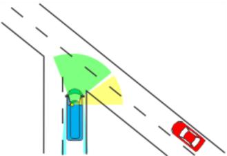
By turning the head to the left 90°, the driver has visibility on the left side only as far as the left door window allows.
