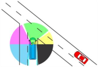
It is physically **impossible** for the driver of a commercial vehicle to secure himself from the right side from this angle.
