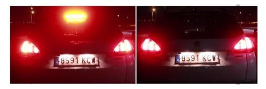
In the Opel Mokka, the brake lights at the ends of the car have a lower light intensity than the 3rd brake light, barely visible, and in combination with the signaling, the distinction between the 2 light is almost zero.
