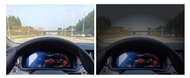
If the electronic display is outside the driver's peripheral visual field, in the middle of the dashboard, or below it, the driver will lose all visibility of the road, because the road will be on the periphery of the peripheral visual field.
