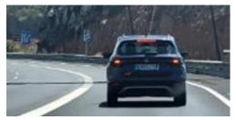
As can be seen, the lights of this braking vehicle can barely be seen due to the too small lighting surfaces. If the image had the sun behind it, or in the driver's field of vision, the brake lights would not have been noticed.
