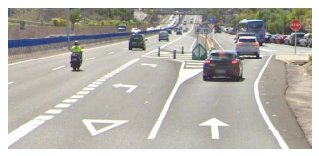
The deceleration lane (right) has the sign and marking Stop, to give priority to another entrance to the highway, and the acceleration lane (left) is blocked by bollards that do not allow further acceleration and do not overlap with the next entrance into the highway.
