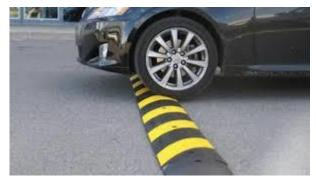
compression, upon entering the surface of the speed limiter, decompression when the wheel reaches the crest, when following the slope and the second compression when the wheel reaches the road side again.
