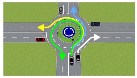
intersection before the exit should change the second lane (inner lane) with the first lane (outer) and exit from the roundabout, without conflicts with vehicles from first lane, as those in first lane were forced to exit at the previous exit.
