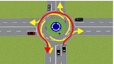
The laws of physics tell us that smooth traffic should avoid stops, and the roundabout was designed as a road node to avoid stops. For this, once you have entered the roundabout, you should have the transit of the roundabout without stopping and without intersecting with other vehicles traveling in other lanes.
