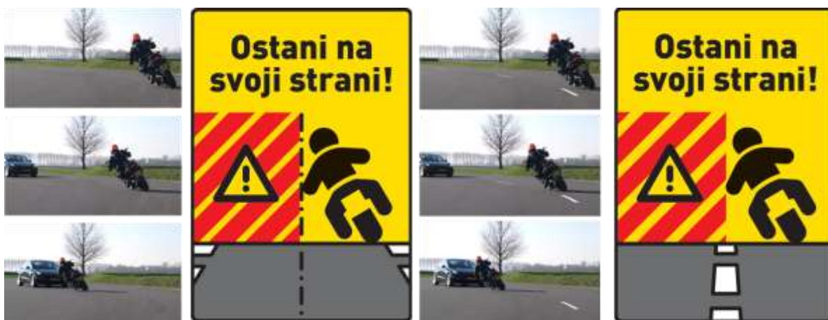
Figure 10 – Design of the information sign “Stay on your side” (for roads with or without a centre line).
