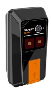
This device has a light to visually warn drivers of the cyclist's presence, a camera with a microphone to record everything that happens during the journey, an App linked to the device and a connection to the DGT 3.0 cloud.
