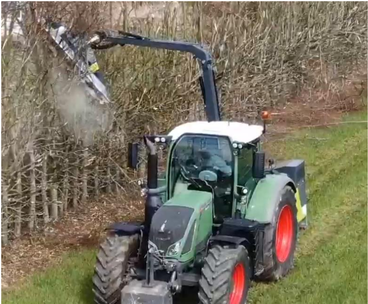
Figure 7- Example of a machine for cutting vegetation in the service of road maintenance
