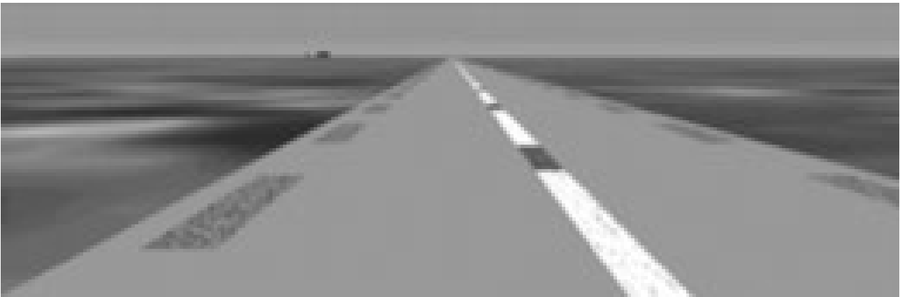
Figure 2.13: Low visual-contrast edge line marking
