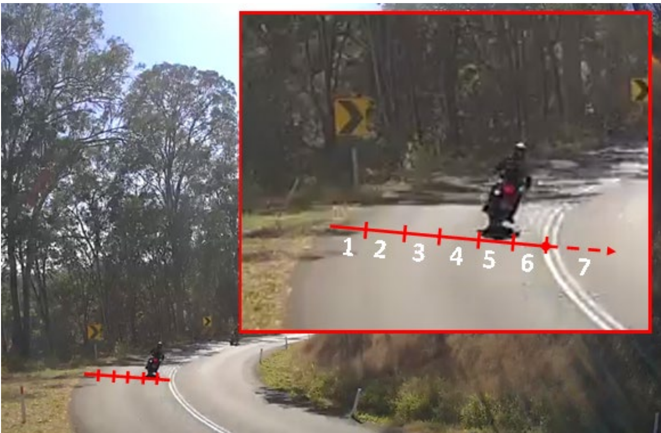
Figure 4.5: Example of reference grid used for measuring the motorcycle lane position at the apex of the trial sites (Site C_1)
