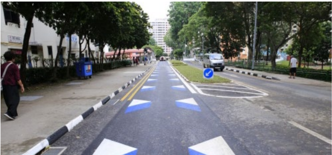
Figure 2.21: 3D transverse line markings used for traffic calming in Singapore
