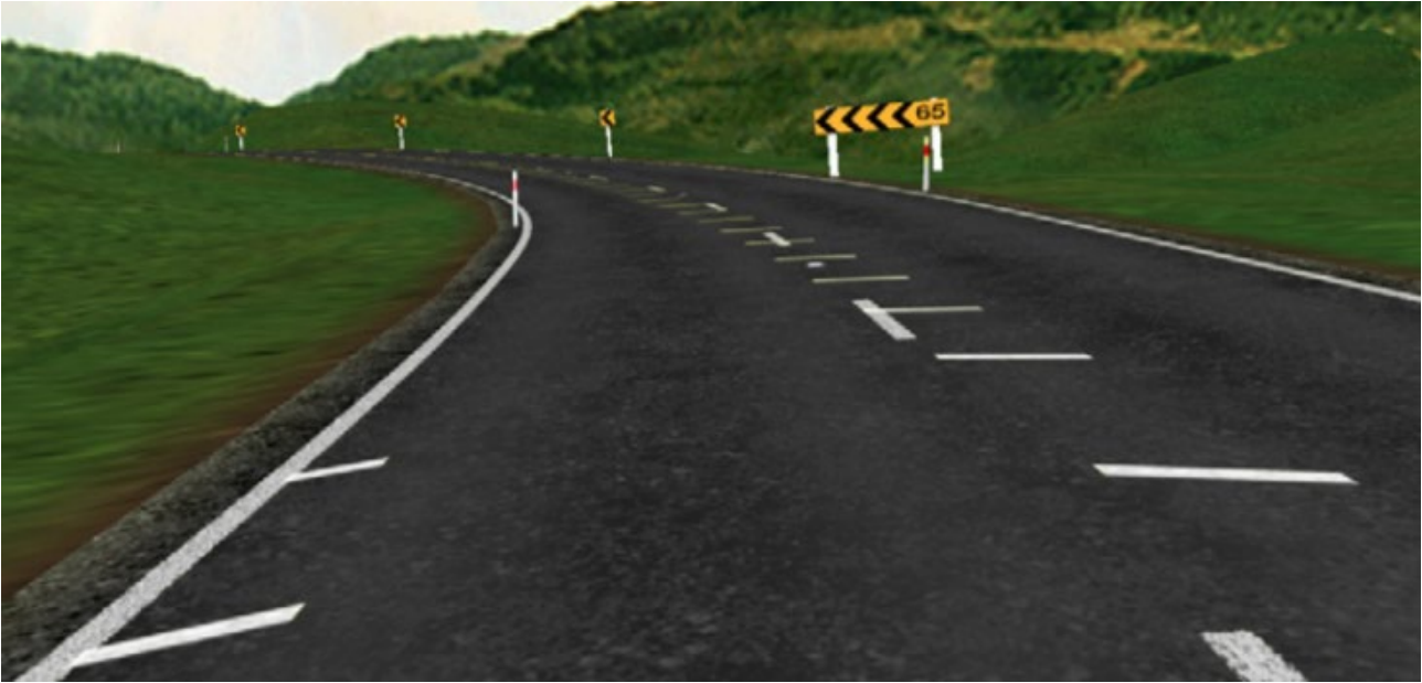
Figure 2.12: Simulated herringbone peripheral line marking and warning signs
