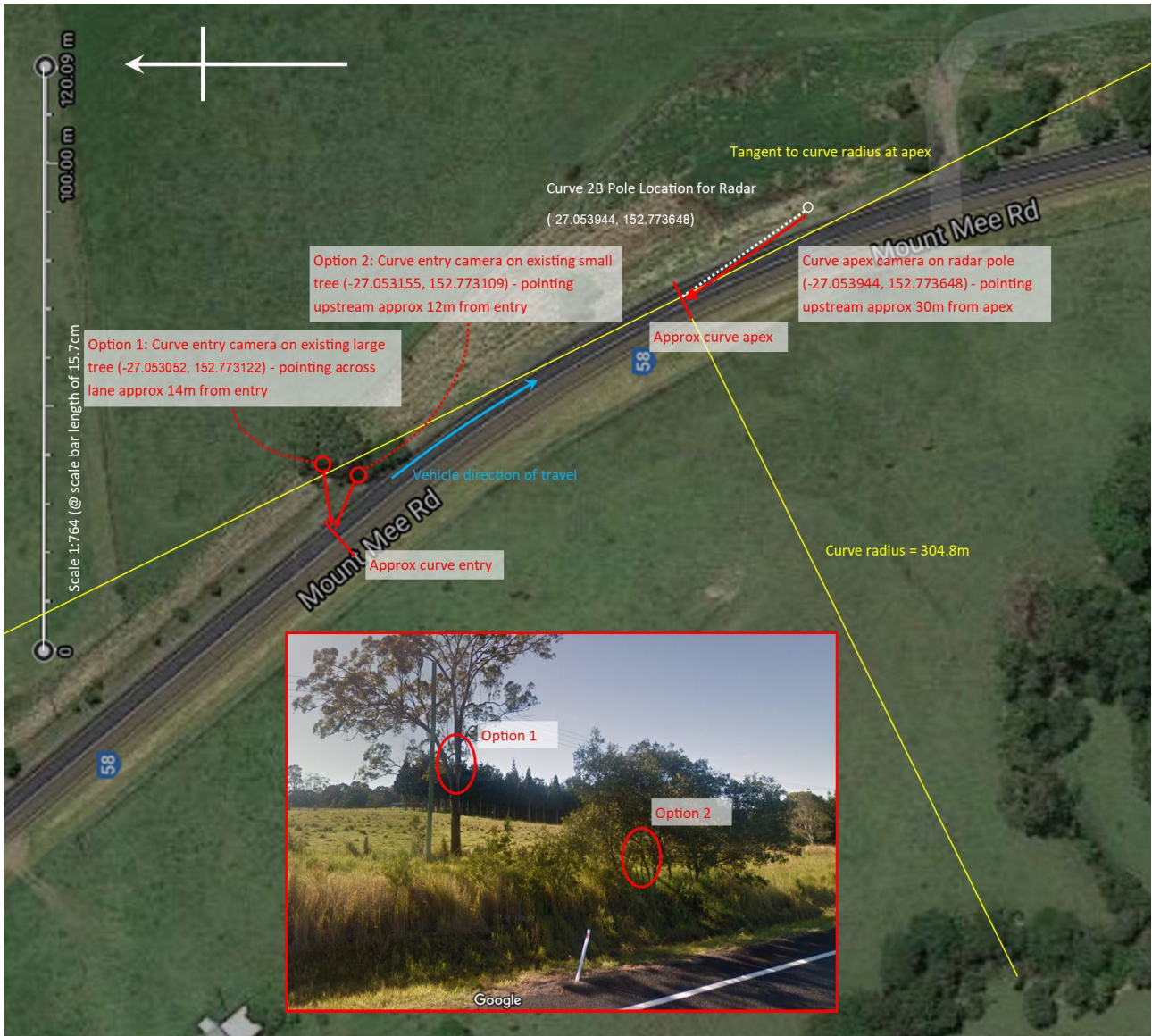
Figure D.4: Locations of radars and video cameras at the shallow trial curve – Control site
