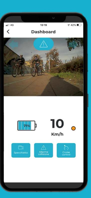
The rear view camera works as electronic mirror to avoid cyclist to turn and lose attention
