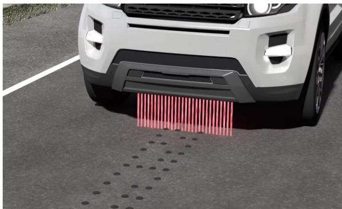
**Fig. 7.** Proposed 32-element linear array.
