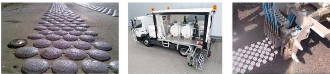
**Fig. 1.** Structured landmarks and a two-component cold-plastic printing machine.
