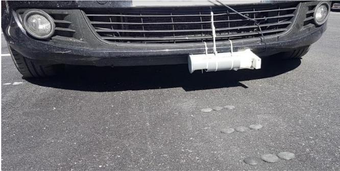
**Fig. 11.** IWR6843AOPEV sensor tested in real scenarios.
