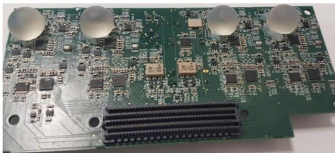
Fig. 3. Four-radar sensor prototype
