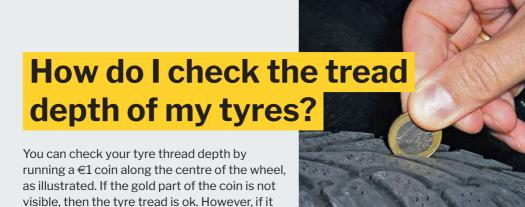
checked. **The minimum permitted tyre tread depth is 1.6mm**. Tyres also have a 'tread wear indicator' block set into them at a depth of 1.6mm. You should check this block to ensure that this indicator is not at the same level as or lower than the tyre tread.
