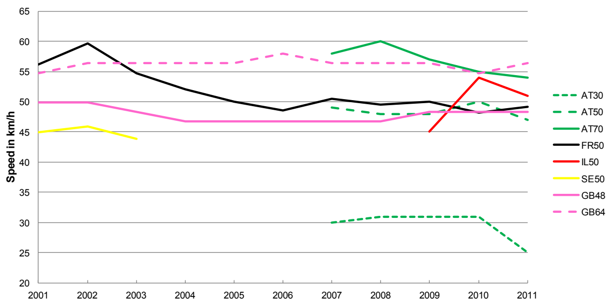
Fig. 9 Mean speed (in km/h) of goods vehicles over 3.5 tonnes, measured in free flowing traffic, on urban roads in some European countries.
